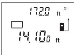
Afterwards, measure the length and the width, one after another, in the same manner as a length measurement. The laser beam remains switched on between both measurements.
