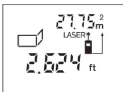
Now, measure length **B<sub>2</sub>** of the second wall. The individual measuring value indicated at the bottom of the display is added to length **B<sub>1</sub>** and the sum of both lengths is multiplied with the stored length **A**. The total surface value is indicated at the top in the display.
