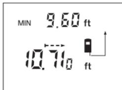
During the measurement, the current length measurement value is indicated at the bottom of the display.
