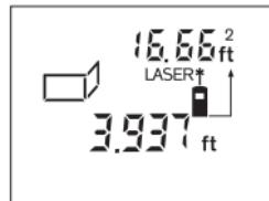
Afterwards, measure length **B<sub>1</sub>** of the first wall. The surface is automatically calculated and indicated. The last length measurement value is indicated
